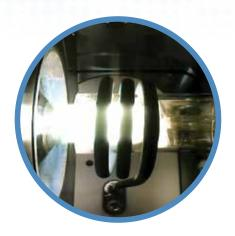
Plasma camera collects HD images of the plasma during all stages of operation, for clear visibility of sample introduction.
