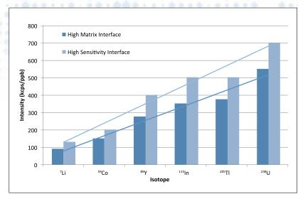
High plasma stability even in 100% organic solvents and low ion energy spread for optimal ion focusing, transmission and sensitivity
