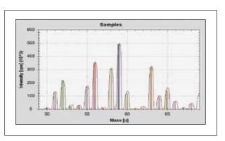
Universal interference removal with He KED, molecular interferences from the matrix are effectively removed whilst maintaining high analyte sensitivity (typically > 40 kcps/ppb Co).
