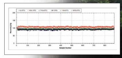
Internal standard recovery over 15 hours of uninterrupted analysis according to EPA Method 200.8.
